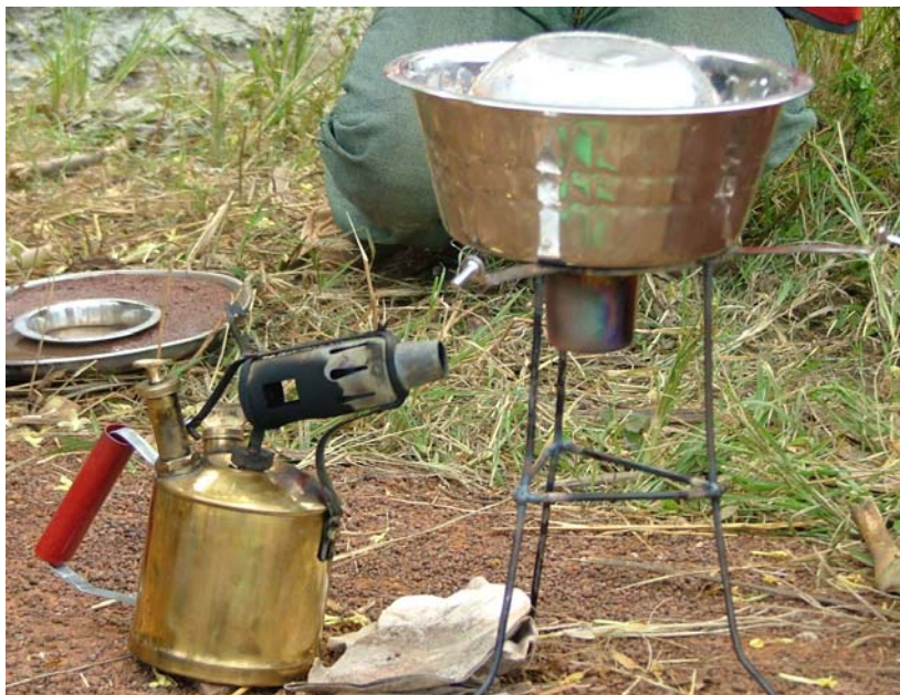
Figure 7: A locally fabricated retort
